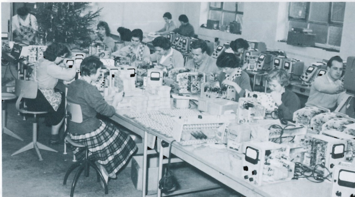
Christmas Season of 1959 at Boeblingen, West Germany, saw the company's first international manufacturing operation—indeed its first such facility outside of Palo Alto—well underway. Products assembled there initially were vacuum tube voltmeters and audio oscillators. European sales grew rapidly with their local manufacture.
