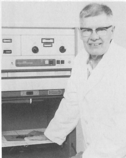
The HP Faxitron 43805 was the "camera" used by Al Duggan of the McMinnville Division to make the X-ray pictures on these pages. (For photography buffs interested in details, he used an Eastman 8x10 LP4 graphic-arts film for his negative, then increased or decreased the contrast as necessary during development).
